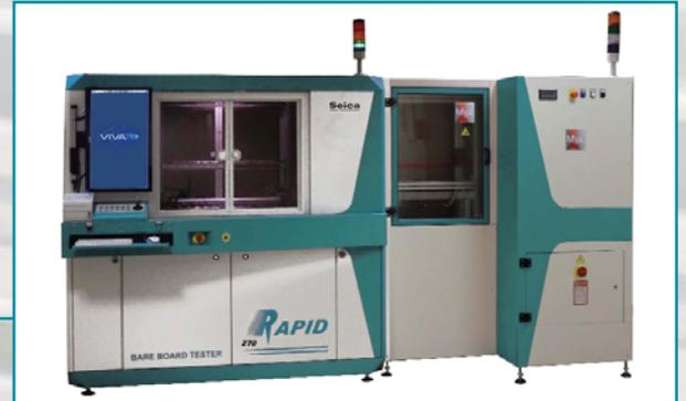
The Rapid 270 combines the versatility and reduced footprint of a vertical system with the automation featuring the testers with horizontal architecture.
