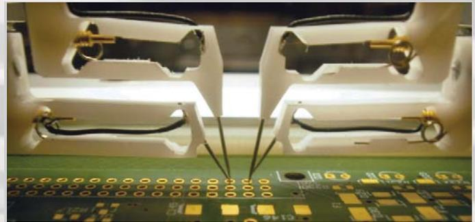
**Barrel Test:** performs continuity and parametric test for the vias of the PCB, which can be determined due to the capability of simultaneous positioning two probes on each side.
