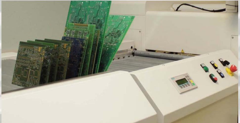
The loading/downloading is performed on the right side of the system and the boards will be automatically divided according to the test result: on the left those with "pass" result and on the right the boards with "fail" result. Both systems provide the opportunity to install a labeling module to apply a label with barcode on the failed boards.
