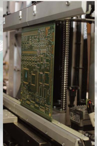
**4 or 8 independent flying probes and a complete range of measurement techniques. Through Seica architecture flexibility all unique market segments can be easily addressed due to the advanced hardware and software integration.**
